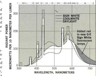
used in them had more red and green energy than, for example, either cool white or daylight lamps. The plastic signs do. And the spectral distribution of the fluorescent sign lamps as compared to cool white and daylight fluorescent lamps shows the effect graphically. These new lamps are designed for 800 ma. operation. Nominal watts range from 35 to 110. Your G-E lamp agent can supply you with prices.
