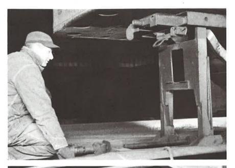
The trailer is held in position on the flatcar by sturdy, but adjustable equipment. At these tie-down points, workmen must see clearly. Getting needed light from stationary units alongside the tracks is the problem in the freightyards.
