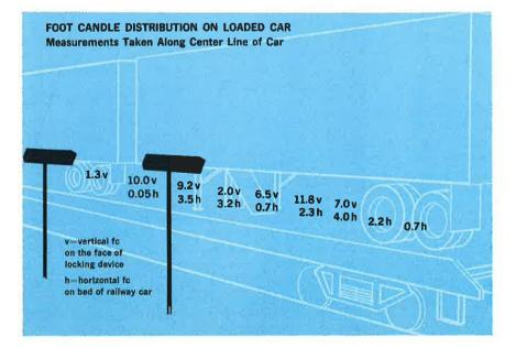
Fluorescent lamp luminaires are spaced about 20 feet apart. Lamps are about six feet above ground level so that light can be directed to the underside of the trailers. The first one is mounted about four feet from the ramp and the units are spaced evenly along the tracks.
