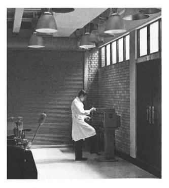
The effect of sunlight (simulated by a row of 1000-watt R-60 Quartzline lamps) through fenestration can be demonstrated here, also. Note that the work is in shadow, and that brightness contrasts are extreme—and uncomfortable.
