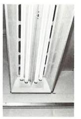
This fixture was designed at Nela Park, and is now available from several manufacturers. It has four high-output lamps, each eight feet long. There is an upward light component and 35° shielding. Light output is high — resulting in lower initial cost. Low operating costs result from the long life and good maintenance characteristics of the high-output lamps.
