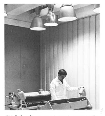
With all of the lamps — color-improved mercury, Lucalox, and De Luxe White Mercury — operating in the same room, the lighting level is 650 fc. However, it can be shown, that where work surfaces are specular, and where long hours are involved, high-intensity sources are not advisable.
